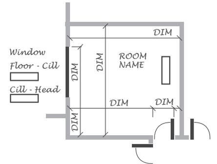
"The best way to provide the required information is to dimension the hallway and landing of the property, this provides a bench mark for us to set all the other rooms from.
