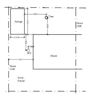
Add the heights and widths externally along with boundaries and any drain details.
