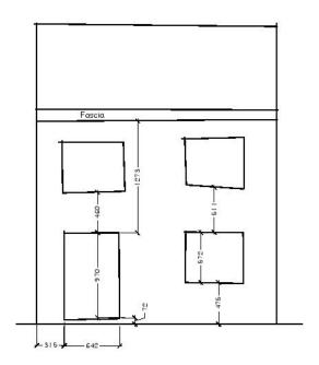
If you intend to have a Dorma or change the roof then draw the elevations adding the heights and widths externally. Again, simple squares for windows and lines for the fascia, the main thing we need is the measurements.
