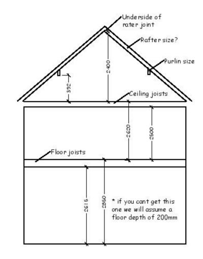
Add the room heights for all levels and measurements in the loift space. Also include the current loft access point .
